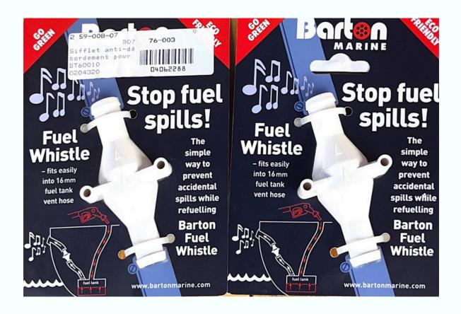
The Barton marine fuel whistle helps to prevent spills when filling a boat's fuel tank. It is installed on the vent pipe and makes a whistling sound while fuel is entering the tank. When the tank is almost full, the whistle stops, showing that you should stop filling.
